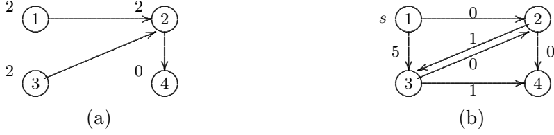
Figure 2: (a) \mathcal{T}_t in (\mathcal{N}, \mathcal{A}) and (b) (\mathcal{N}, \mathcal{A}) with reduced costs
