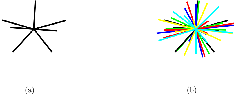
Figure 4: Seven equally spaced non-coplanar orientations – 4(a) and set of six initial points with seven equally spaced non-coplanar orientations – 4(b).
